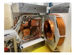
A cyclotron is a particle accelerator machine that uses electromagnetic fields and RF signal to propel charged particles to very high speeds and energies, used to produce radioisotopes, such as 18F, which are essential / core components of radiopharmaceuticals.
